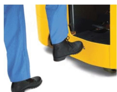
Travel and lifting are stopped when the operators leaves the compartment
