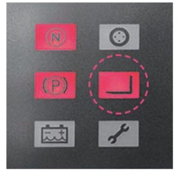
The lifting work interlock is displayed on the monitoring
