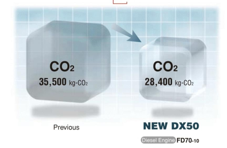
Komatsu tested data, comparison with FD70-8 model.
